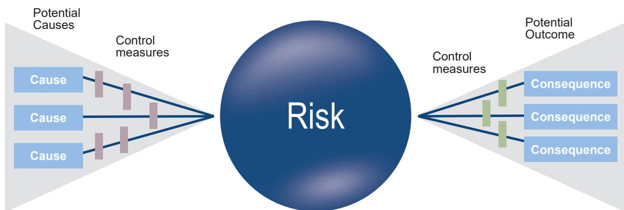
Figure 9. Bow-Tie Diagram Shows Risk Causes, Control Measures, and Consequences
